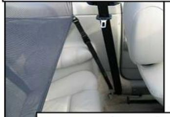
STEP 5: NEXT ATTACH THE SILVER HOOK TO THE SEATBELT ROD NEAR THE FLOOR. MAKE SURE YOU ATTACH THE HOOK BEHIND THE RUBBER BUMPER SO IT DOES NOT INTERFERE WITH THE SEAT BELT (REPEAT ON THE OTHER SIDE)
