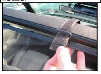
STEP 2 CONT: PULL THE STRAP SNUG AND THEN FOLD OVER THE STRAP SO THE VELCRO ON EACH SIDE OF THE STRAP IS HELD IN PLACE
