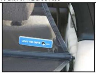
YOU MAY NEED TO ADJUST THE TOP STRAPS ON THE ROLL BAR TO REMOVE SOME OF THE WRINKLES
