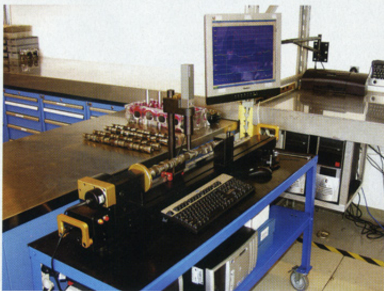
The doctor is in. Skunk2 uses a cam measurement doctor to check profiles on their cams to ensure quality. The cam doctor can measure differences to within 0.000001 inches between each lobe.
