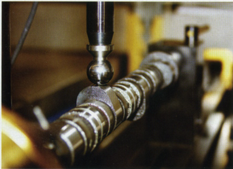
The doctor is in. Skunk2 uses a cam measurement doctor to check profiles on their cams to ensure quality. The cam doctor can measure differences to within 0.000001 inches between each lobe.
