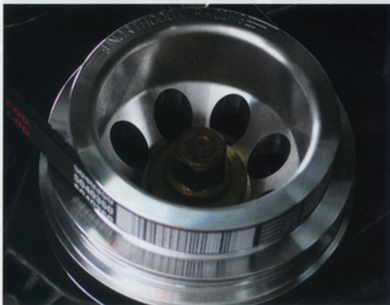
The UR pulley set made an improvement of 3.0 peak horsepower but gains as high as 5.0 horsepower can be realized.
