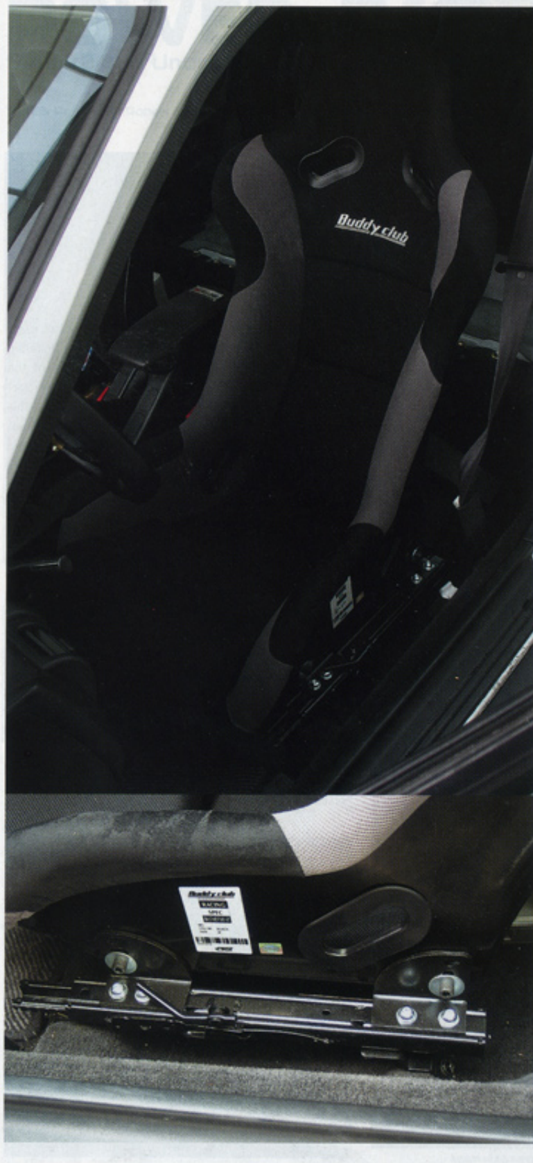
Keeping the driver secured in place at the track is a Buddy Club bucket seat mounted on Bride seat rails.
