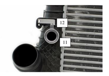
13. Install your new Turbosmart BOV assembly in this orientation. Ensure that O-ring (39.00x2.00) is in place before placing the BOV assembly on the adapter. Secure your new Turbosmart BOV with the V-band clamp. Ensure that the V-band clamp is secured tightly.
