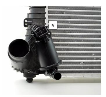
**10.** Remove the BOV chamber by turning it upwards. The BOV chamber should just unscrew.
