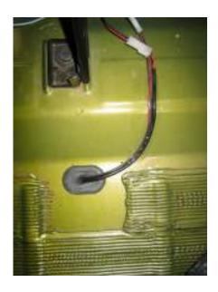
8. Mount the door sensors to the inside door frames. Use the stick pads provided. Mount the sensor just underneath the door latch. Route the wires around the body seam. Place a small piece of electrical tape on the body seam. Wrap the wire over the top of the tape towards the inside of the cab then secure the wire with another piece of electrical tape.
