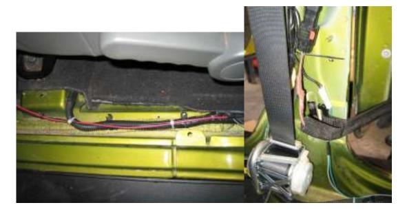
10. Route the system disable switch, POS+ and NEG- wires up the driver side to the "A' pillar on the front diver side door. Remove the side dash panel. Drill a hole in the dash to accommodate the switch. Run the three wires for the disable switch through the dash and plug into the back of the switch. Mount the ground from the plug to a metal surface for the switch illumination.
