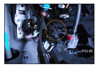
Step 4- Double check to make sure the red tab is in the unlock position on the grey connector. Now plug the OEM harness into the Sprint Booster.
