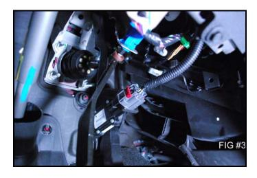
Step 5- You can now lock the harness connection by pressing downward on the red tab. You should hear it click in place. If the connection is not solid or the tab does not click back in place – the harness can easily come off the Sprint Booster.
