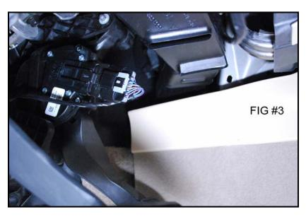
Step 4- Once the Sprint Booster connection is finalized, relock the grey clip back into place.
