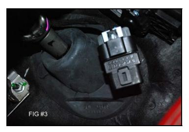
Step 3- Proceed to re-connect the harness, with Sprint Booster, into the pedal with the same precaution mentioned as Step 2. Make sure your OEM harness will have enough slack before reconnecting with the Sprint Booster fully installed. The harness may require a new route to give the needed freedom in the harness.
