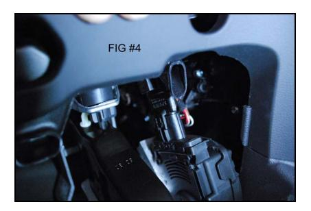
You may find the heating vents to obstruct the alignment of the Sprint Booster. The vents will move a bit to one side.
