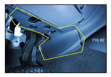
The highlighted shroud will remove with little effort, no tools are needed, a healthy downward pull will release it of its holding clips.
