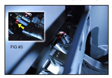
The red tab acts as a locking device for the connector to stay attached. Unlock the connection by pressing the red tab upwards.
