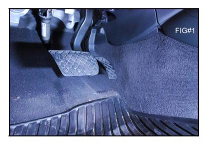
Step 2 – Remove the upper part of the cosmetic cover along the lowest part of the dash that is just above the gas and brake pedal. Shown more in Fig #2. It will not need to be totally removed, it only has to hang loose for the install of the Sprint Booster.
