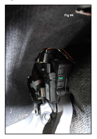
Step 4- The factory connector should now be free, you can proceed to put in the Sprint Booster. Match up the notches/clips on either end of the Sprint Booster, then clip it into place. Be sure to have your pins aligned before inserting, bent pins will cause the plug to malfunction. The Sprint Booster will only slide in place easily one way. Proper install is shown in Fig #5
