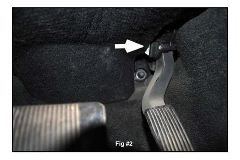
The carpet that is on the left side of the gas pedal will have to be held back in some way to access the top of the pedal and the harness while installing the Sprint Booster. You can just push it upwards with minimal effort by hand.
