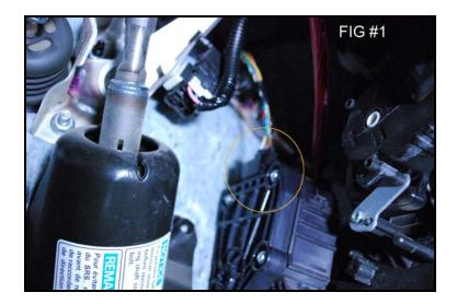
Step 2 – Where the wires meet the plastic connection you will feel a tab on the right side when looking at it from the drivers position. Squeeze the tab while lifting upward to release the connection. The Sprint Booster will install between this connection.
