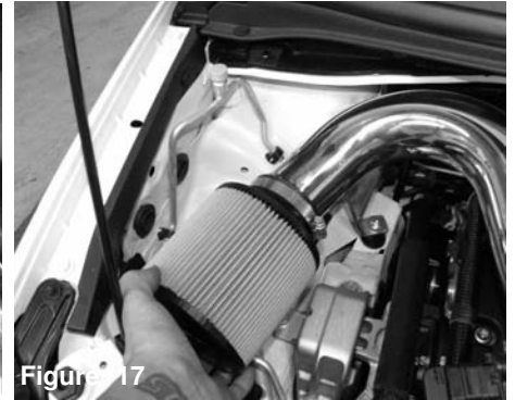
Figure 17 Install the air filter and tighten using 8mm nut driver.
