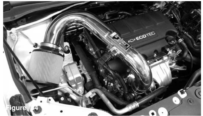
Figure 4 Congratulations! You have just completed the installation of this intake system. Periodically, check the alignment of the intake, normal wear and tear can cause nuts and bolts to come loose. Note: Check clearance and adjust if needed! Failure to check the alignment and adjust the intake can cause damage that will void the warranty. Injen Technology is not responsible for any damages caused by/from improper installation.
