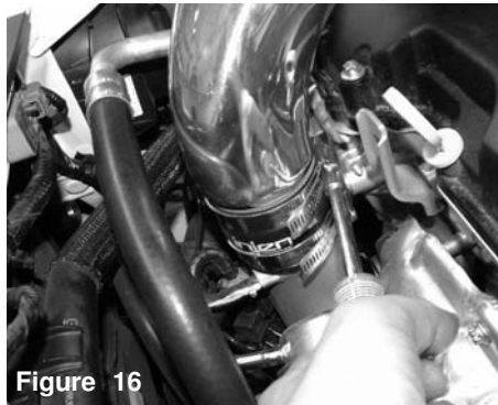
Figure 16 Tighten the clamp on the turbo using 8mm nut driver.
