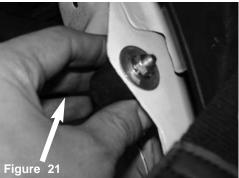
Secure the vibra mount using M6 nut and washer.
