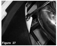
Tighten both nuts on vibra mount using 10mm wrench.
