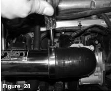
Position the intake for the best fit and tighten clamp on hose usign 8mm nut driver.
