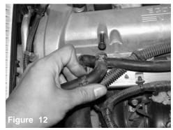
With pliers pull back crank case line from engine.
