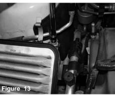
With 10mm socket and ratchet, loosen and remove the bolt holding in A/C line and air box.
