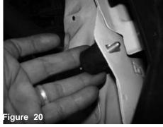
Attach the vibra mount to the front of the vehicle on square hole cut out on radiator support.
