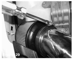
Install the high flow filter to intake tube and tighten using 8mm nut driver.
