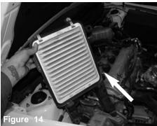
Carefully manuever the bottom half of air box out of vehicle. Note: becarefull and not damage the A/C line. Re-install the bolt from previous step and secure the A/C line.
