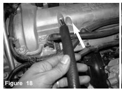
Attach the provided 10mm hose to the engine.
