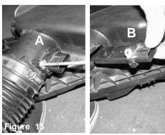
A) With phillips screwdriver loosen the 2 screws holding in MAF sensor.
