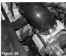
Tighten the clamp on throttle body using 8mm nut driver.
