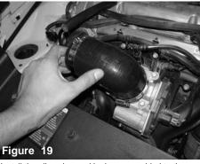
Install the elbow hose with clamps provided to the throttle body. Make sure the short side of hose is on the throttle body.
