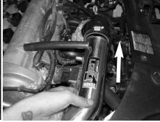
Install the intake asembly into the vehicle and position to hose.
