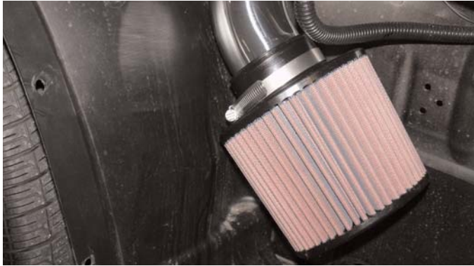
Press the Injen filter over the end of the intake and tighten the clamp on the filter neck.
