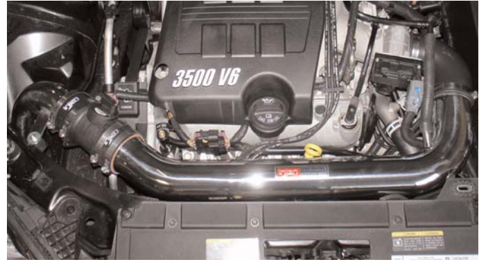
Align the entire intake for best possible fit. Once proper clearance has been made through out the length of the intake continue to tighten all nuts, bolts and clamps. Replace the bumper back to its original location and reconnect the negative battery terminal. Congratulations! You have just completed the installation of this cold air intake system.
