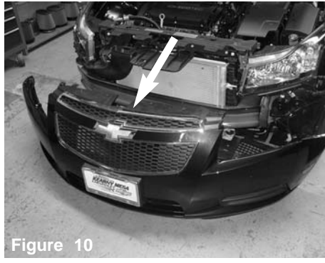
Figure 10 Carefully remove the bumper cover, this requires 2 10mm bolts on top, push-clips, and t-25 screws located on the bottom of the vehicle. This is required for the cold air installation.
