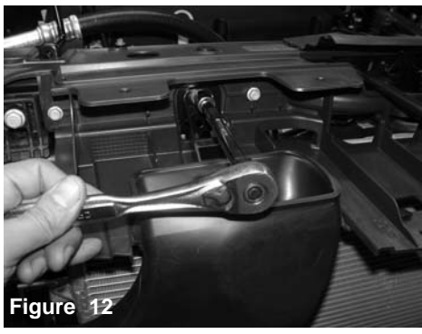
Figure 12 Loosen the bolt holding in the air box snorkel using 10mm socket and extension.
