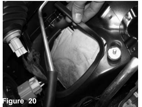
Figure 17 Remove the 2 clips holding in the plastic auxiliary inlet.
