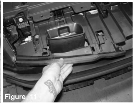
Figure 11 Remove the air box snorkel guard from the vehicle.
