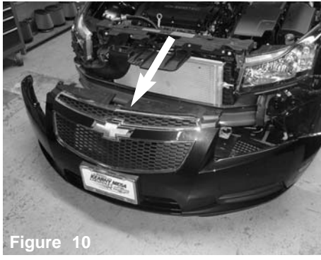
Figure 10 Carefully remove the bumper cover, this requires 2 10mm bolts on top, push-clips, and t-25 screw located on the bottom of the vehicle. This is required for the cold air installation.
