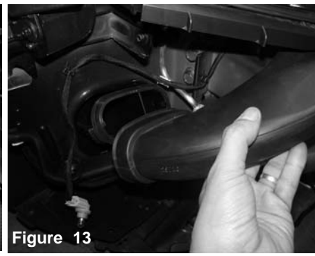
Figure 13 Pull back the air box snorkel from the resonator.
