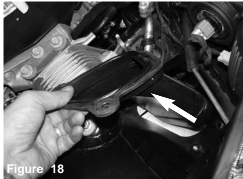
Figure 15 A) Push back resonator from grommets on frame B) Roll back resonator into the splash guard to remove. Note: some force me be required to remove.
