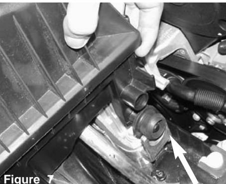
Figure 7 Pull back the grommet from the bottom of the air box.
