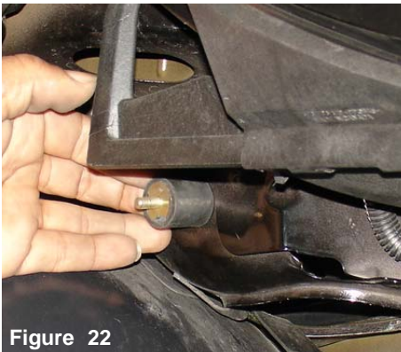
Figure 19 The male/female vibra-mount is aligned and screwed over the air box stud.
