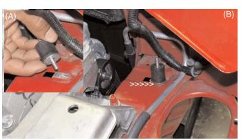
Remove the 6mm bolt (A). Place the vibra-mount with the fender washer into the pre-tapped hole and turn the vibra-mount into the tapped hole until it bottoms out (B).
