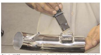
Take the MAFS removed earlier from the stock air intake box and press it into the machined adapter. Use the stock sensor screws to reattached the MAFS into the machined adapter.
