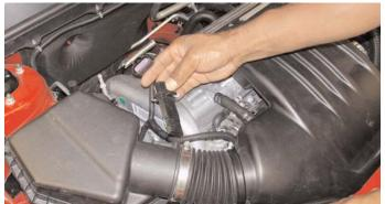
Remove the mass air flow sensor from the stock air intake box. Set the sensor to one side to be used later in the instruction.
