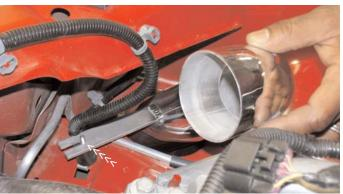
Once the secondary intake has been inserted into the resonator opening align the bracket to the vibra-mount stud.
