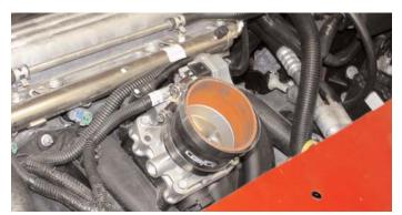
Press the 2 3/4" x 3" step hose over the throttle body and use two clamps on the hose, tighten the clamp on the throttle body at this time.
