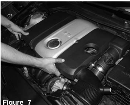
Figure 7 Carefully lift and pull up on the factory air box/engine cover and remove it from the engine.
