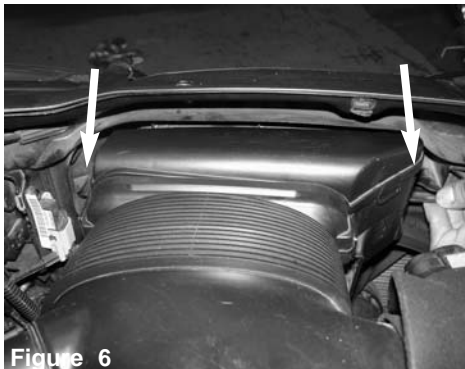
Figure 6 With T25 torx key, loosen the 2 screws holding in factory ram-air unit attached to the radiator support.
