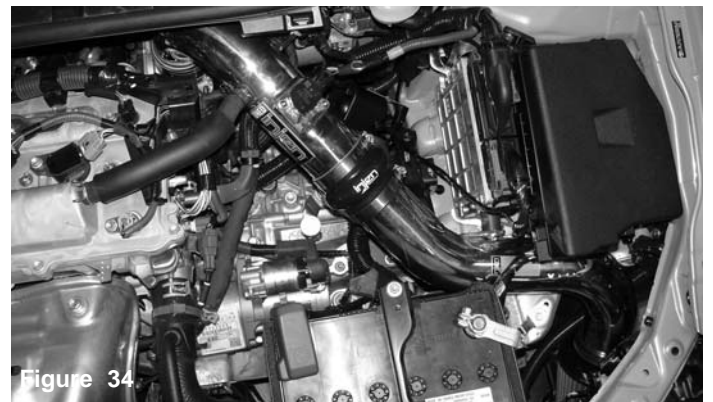
Figure 32 Tighten the clamps on the hump hose using 8mm nut driver.
