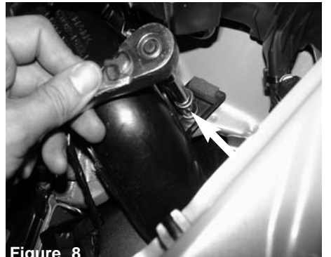
Figure 8 With 10mm socket and extension, loosen the bolt holding in the plastic snorkel assembly.
