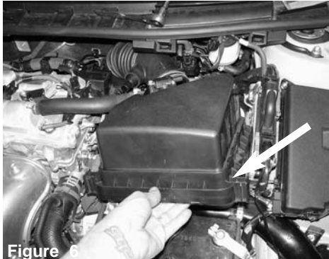
Figure 6 Un-clip the upper half of air box and remove.
