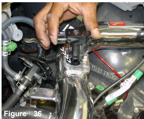
Figure 36 Take the mass air flow sensor and insert it into the machined sensor adapter. Use a dab of light oil on the O-ring, this will insure a good seal.
