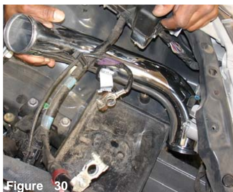
Figure 30 The air intake tube is lowered it into the engine compartment and into the resonator opening, align the intake bracket.
