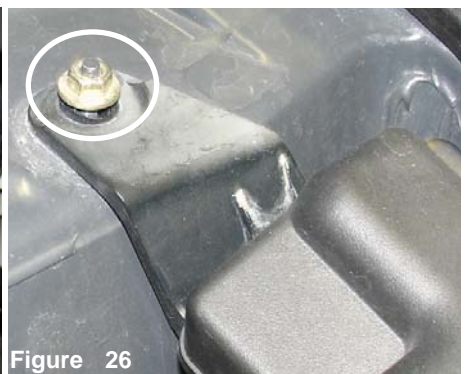
Figure 23 Remove the m10 bolt that secures the fuse box to the fender wall.
