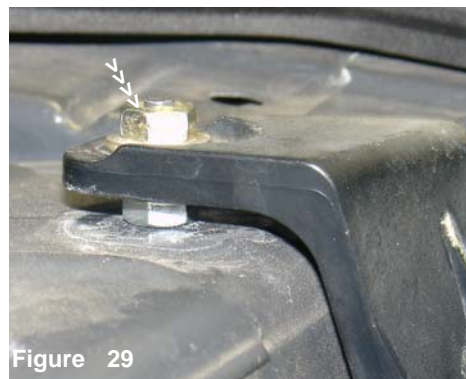
Figure 29 Secure the fuse box by using the stock m6 flange nut as shown above.
