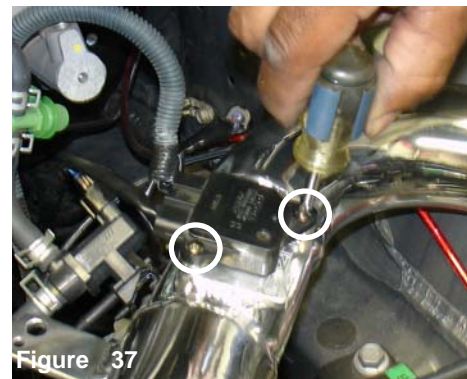
Figure 37 The stock bolts are used to fasten the mass air flow sensor to the machined sensor adapter.
