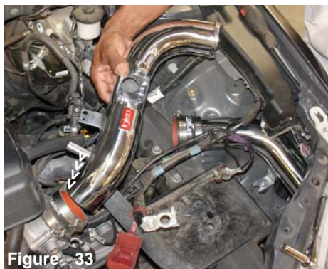
Figure 33 Lower primary intake into the engine comartment. Press the top end of the intake into the throttle body step hose.
