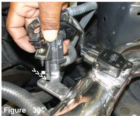
Figure 39 The vacuum switching valve locating pin is now pressed into the flat intake bracket.
