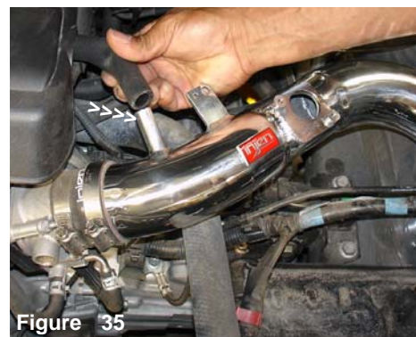
Figure 35 Press the other end of the 17mm heater hose over the intake port as shown above.
