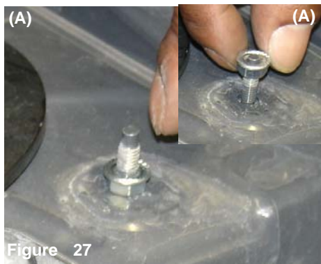
Figure 27 Take the m6 flange nut in this kit, place over the top of the stud (A). Screw the nut all the through until it bottoms out as shown above (B).
