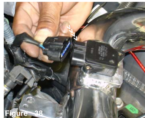
Figure 38 Press the electrical harness clip to the mass air flow sensor until it snaps in place.
