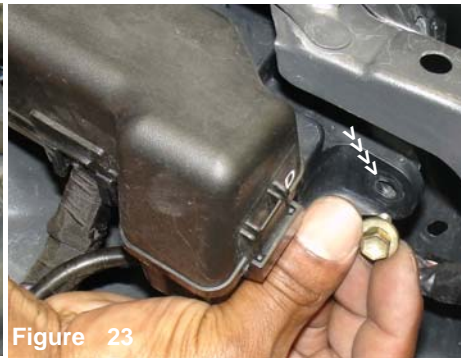
Figure 20 Here is a shot from under the wheel well showing how the vibra-mount is attached.
