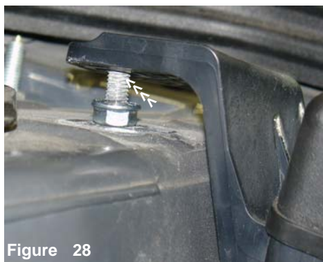
Figure 28 Place the fuse box lip over the stud. The entire fuse box is now raised making room for the air intake.
