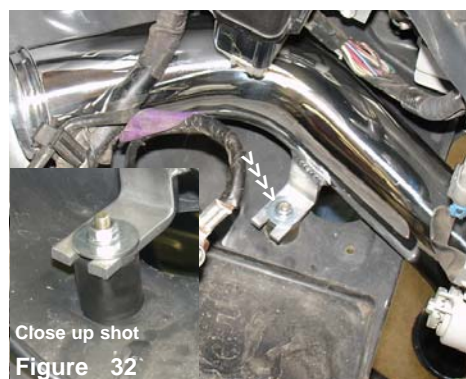
Close up shot Figure 32 The m6 flange nut and fender washer is used to secure the secondary intake.
