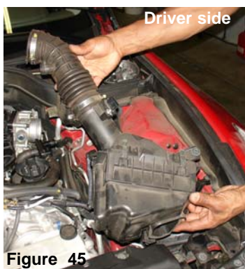
With the harness and bolt out of the way, continue to pull the entire air box cleaner and air intake duct from the engine compartment.
