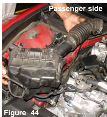
With the harness and bolt out of the way, continue to pull the entire air box cleaner and air intake duct from the engine compartment.
