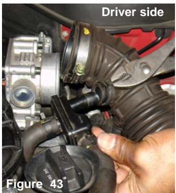
Once the CCV box has been remove, continue to detach the air intake duct from the throttle body.
