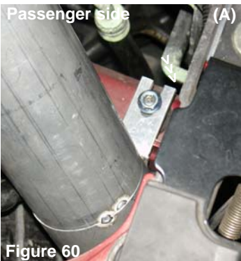
Place a fender washer over the intake bracket, use the m6 flange nut to tighten the air intake bracket to the stand-off s shown in figures (A) and (B).
