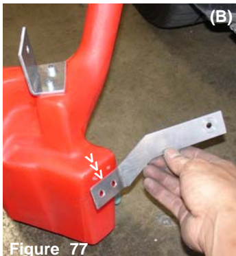
Figure 76 Figure 77 Use the m6 x 12mm bolts in this kit to fasten the bracket to the reservoir bottle (A). The horizontal long bracket is now aligned to the side m6 press nuts (B)
