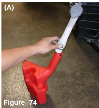
Figure 74 Figure 75 The top spout is aligned to the spout on the reservoir tank (A). The top bracket is aligned over the press nuts on the top of the reservoir bottle (B). Note: The stock level sensor indicator will not be used for this installation because of the difficulty of cutting out and removing the sensor.
