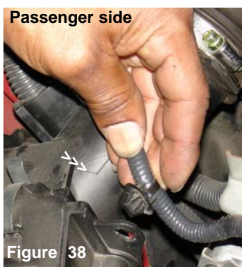
Pull the harness clip away from the top of the air box cleaner,
