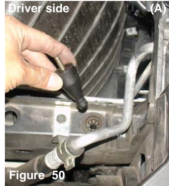
Do the same on the Driver side. Align the stand-off to the stock grommet (A) then push down on the stand-off until it is fully inserted into the grommet(B).
