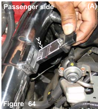
Figure 64 Figure 65 Carefully, insert the mass air flow sensor into the sensor housing of the cold air intake (A). Push until the head of the sensor comes to rest with the top of the sensor adapter. The stock 4mm bolts are used to secure the mass air flow sensor to the sensor adapter (B).
