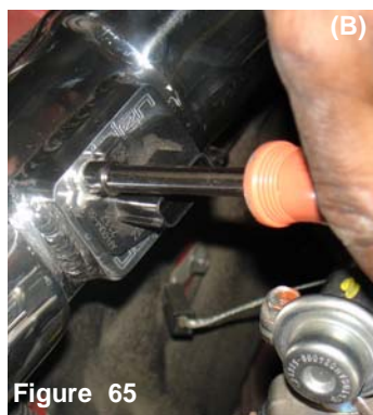
Figure 64 Figure 65 Carefully, insert the mass air flow sensor into the sensor housing of the cold air intake (A). Push until the head of the sensor comes to rest with the top of the sensor adapter. The stock 4mm bolts are used to secure the mass air flow sensor to the sensor adapter (B).
