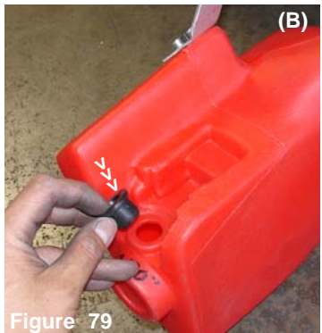
Figure 78 Figure 79 Use the last of the m6 x 12mm bolts to fasten the bracket to the reservoir bottle as shown in figure (A). The grommet that was removed from the stock reservoir bottle is now inserted into the new reservoir bottle (B).
