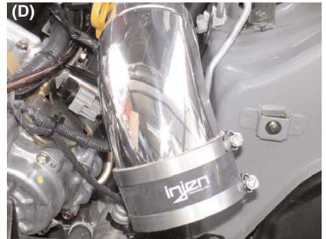
(D) CONTINUING TO INSTALL SECONDARY INTAKE- Press the 3 1/2" straight hose over the end of the primary intake. Use two large clamps and only tighten the clamp located on the end of the intake (D).
