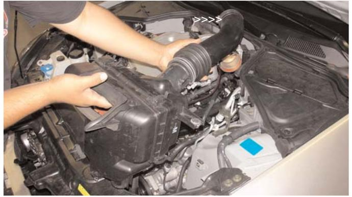
Loosen all clamps and remove bolts that holds the air intake duct and air intake box in place. Gently, remove the entire air box assembly from the engine compartment and set it aside.
