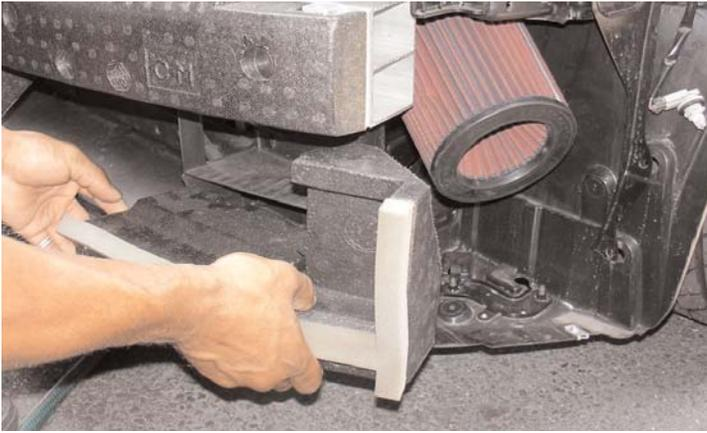
Once a corner section has been cut off, place it in back in the stock location. Cut just enough to give you about 1/4" to 3/8" clearance between the filter and foam insulation. **Direct air to the filter will cause air turbulence that will cause the engine to stall. Do not remove foam insulator from car, must be used.**
