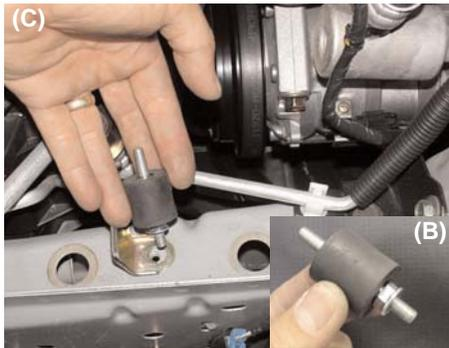
(C) Find the remaining vibra-mount and screw an m6 nut as shown in picture (B) With the m6 nut facing down, screw the vibra-mount into the bracket and frame (C).
