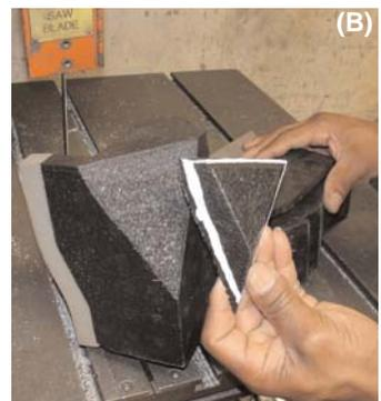
(A) Take the foam insulator located in the front bumper and use a bandsaw, hack saw or saw that is capable of slicing through foam. It will be necessary to cut a corner piece from the foam insulator in order to make room for the filter. Start by cutting about an 1" as shown in figure (A) and (B). **Do not remove foam from the bumper support.**
