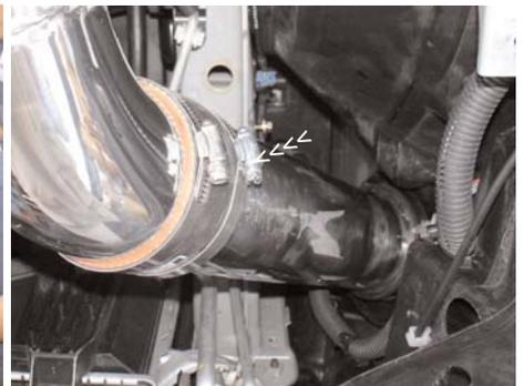
Insert the top end of the secondary intake into the 3 1/2" straight hose located over the primary intake. Semi-tighten the clamp to hold both intakes together.
