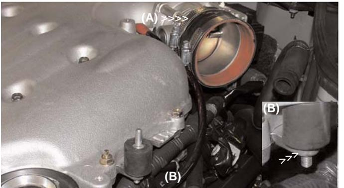
Press the 3 1/8" straight hose over the throttle body and use two clamps on the hose. Tighten the clamp on the throttle body side in order to prevent the hose from slipping off (A). Take the vibra-mount and screw it into the pre-tapped wing located to the side of the intake manifold cover (B). Vibra-mount fully installed (C).
