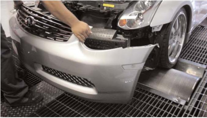
This installation will require the removal of the front bumper. Refer to page three for step by step instructions.
