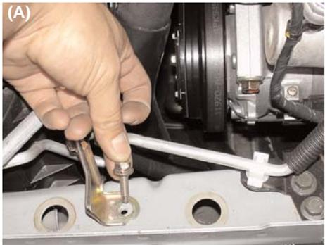
(A) Remove the m6 stock bolt securing the air conditioning bracket to the frame.
