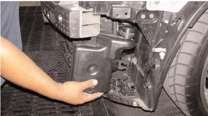
Once the bumper has been removed continue to unscrew the m6 bolt then remove the air resonator box from the driver side bumper. The removal of the resonator box will allow room for the air filter and secondary intake assembly.
