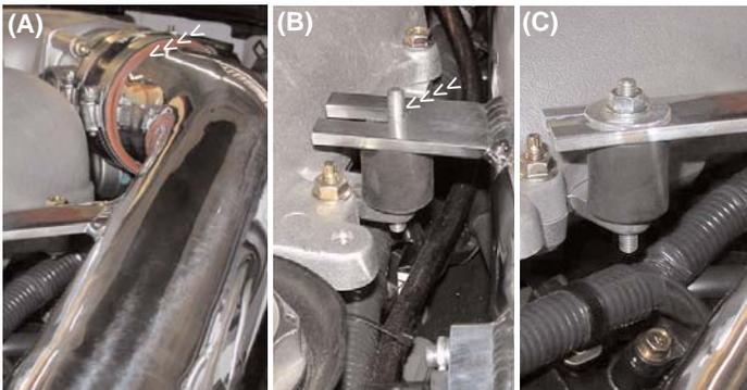
Press the intake outlet into the throttle body hose (A). Align the intake bracket to the vibra-mount stud (B). Place the fender washer over the stud and screw the m6 flange nut on the stud (C).
