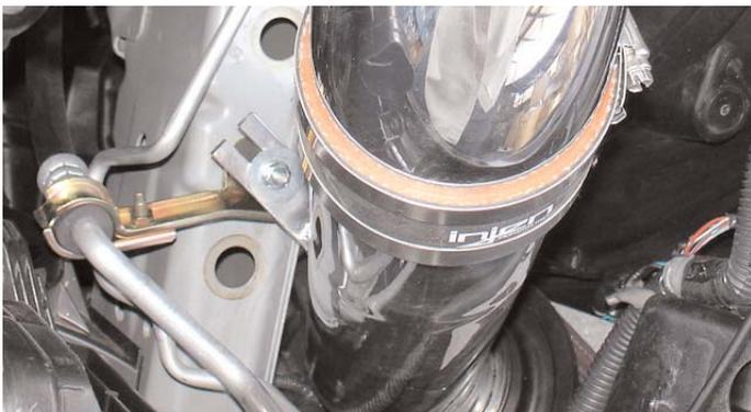
Once the primary and secondary intakes have been aligned and butted together, set the intake bracket over the vibra-mount stud. Use the m6 flange nut and fender washer to secure both intakes in place.
