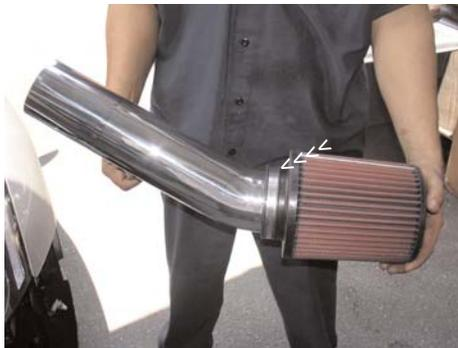
Take the secondary intake and press the large Injen filter over the end of the intake. Once the filter has been positioned in place, fasten clamp located on the filter neck.
