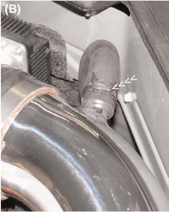
(A) Find the stock breather hose and press it directly over the 1/2" intake port (A). Once the breather hose has been pressed over the intake port, use the stock clamp to prevent the hose from slipping off (B).
