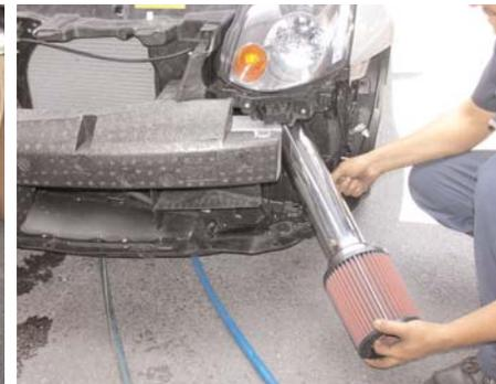
Insert the top end of intake into the driver side bumper and up through the engine compartment.
