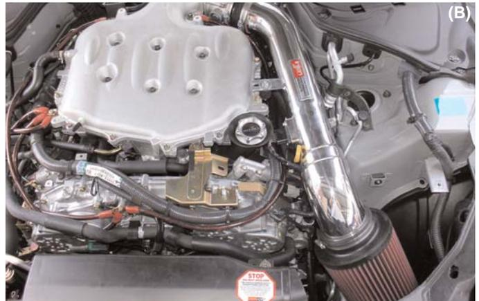
(B) Short ram installation- Press the Injen filter over the end of the intake and fasten clamp located on the filter neck. Align intake for best possible fit. Once fitment has been cleared continue to tighten all nuts, bolts and clamps.
