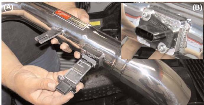
Locate the primary intake and carefully insert the air mass sensor into the machined flange welded to the intake (A). Use the stock screws to fasten the sensor in place (B).
