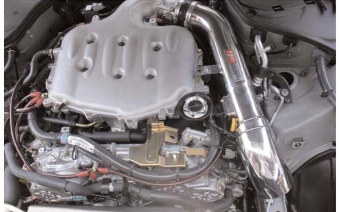
Align the entire intake for best possible fit then continue to semi-tighten nuts, bolts and clamps just enough to hold the intake in place.
