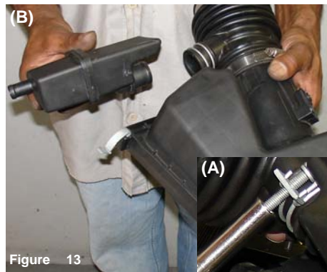
Figure 13 Loosen the clamp on the air intake duct that connects the crankcase vent box (A). Disconnect the CCV box from the air intake duct as shown above (B).
