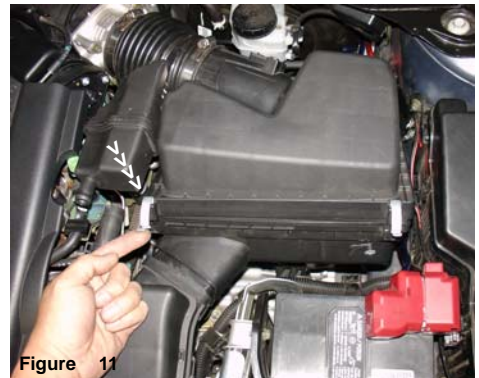
Figure 11 The first metal clip is unsnapped from the lower air box.
