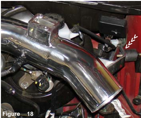
Figure 15 The vibra-mount is screwed all the way until it sits flush with the bracket.
