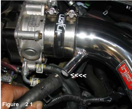
Figure 18 The intake is pressed into the throttle body hose and the intake bracket is aligned to the vibra-mount stud.
