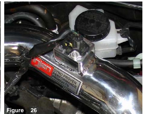
Figure 23 Insert the original mass air flow sensor into the machined billet sensor adapter. To prevent kinking of the gasket, be sure to use a light oil to moisten the gasket.
