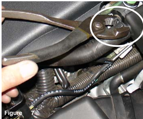
Figure 7 Depress the wire tension clamp on the crank case breather hose and pull it away from the crank case vent box.
