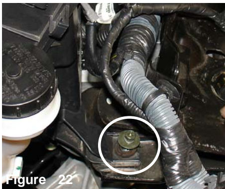
Figure 19 Remove the second bolt (B) from the metal battery tray.
