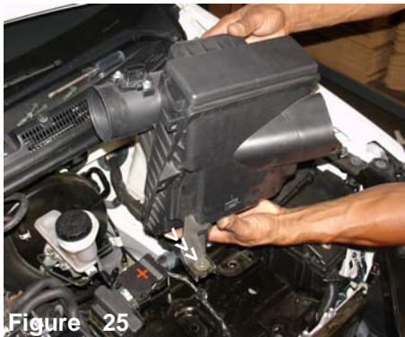
Figure 22 Now that the tray has been lifted out of the way, continue to loosen the m6 bolt located on the corner of the air box.
