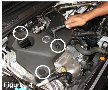
Figure 4 Loosen all three m6 bolts located on the engine cover as shown above.
