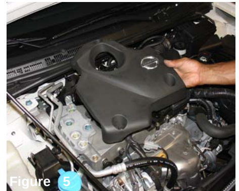
Figure 5 Once all three bolts have been removed, continue to pull the plastic cover out of the engine compartment.
