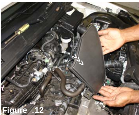
Figure 12 Once the m bolt has been removed and the hose clamp has been loosened, continue to pull the CCV box away from the air intake duct.
