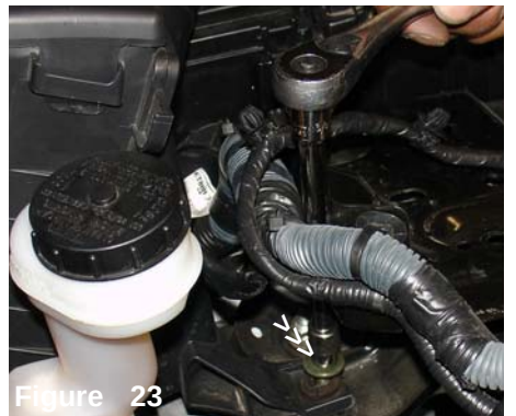
Figure 20 Bolts (C) and (D) are removed next. This will now give you access to the last m6 bolt securing the air box cleaner.
