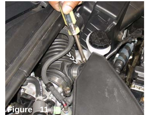
Figure 11 Loosen the hose clamp that fastens the CCV box port to the air intake duct.
