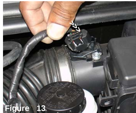
Figure 13 Press the plastic tab on the female connector and pull the electrical harness clip from the mass air flow sensor.
