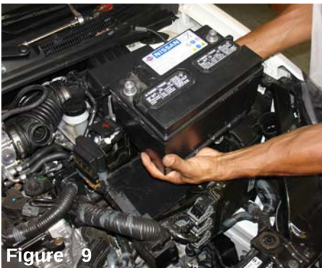
Figure 9 Remove the battery cables and carefully pull the battery out of the engine compartment for now.
