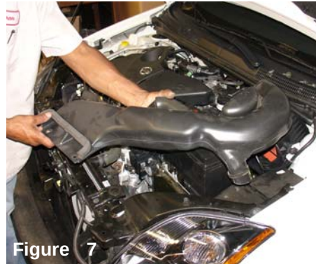
Figure 7 Once you have pulled plastic clips out, continue to pull the factory air scoop out of the engine compartment.
