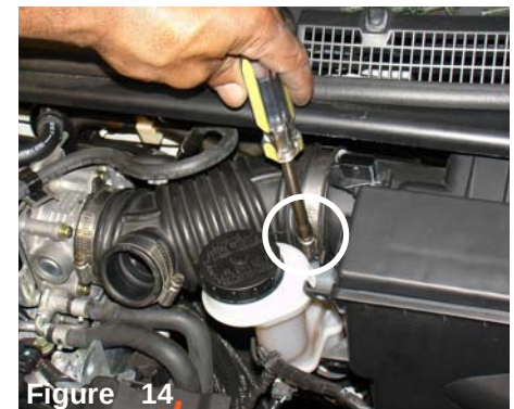
Figure 14 Loosen the hose clamp that connects the air intake duct to the air box cleaner.
