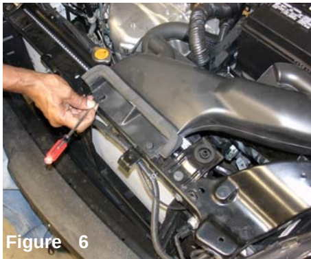
Figure 6 With the use of a screwdriver, insert the head under the clip, pop the plastic clip up and pull the entire clip out.
