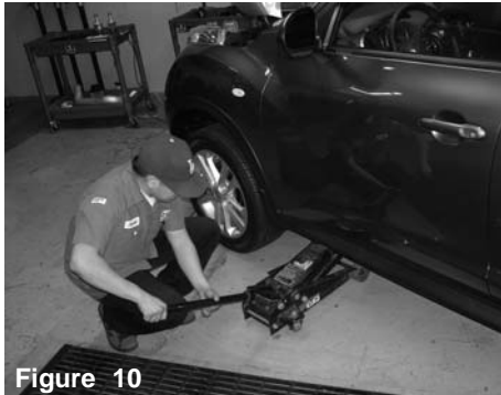
Figure 10 You will need to remove the driverside wheel. Use a jack to lift up the driverside wheel.
