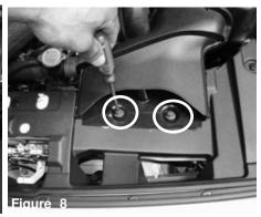
Use a flat head screw driver to pop the plastic clips from the front air scoop.
