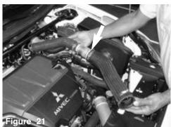
Once you have loosened both upper and lower clamps, continue to pull the intercooler tubing out of the engine compartment.
