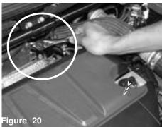
Loosen the clamp on the upper intercooler hose.
