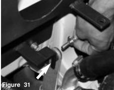
The lower heat shield bracket is aligned to the air box brace. The stock 12mm bolt is inserted into the stock air box rubber vibration mount and into the heat shield slotted bracket.
