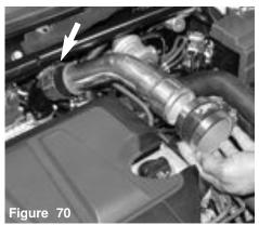
Adjust and semi-tighten the clamp on the tubing. Press the 2 1/2" hose over the opposite end of the tubing. Place two clamps over the 2 1/2" hose. Page 7 of Part# SP1899
