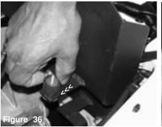
Once the m6 flange nut and fender washer have been semi-tighten under the bracket, continue to turn the vibra-mount until it is firmly tightened.
