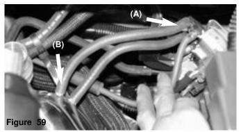
Once the 6  $3/4^{\circ}$  hose has been pressed over the upper solenoid port (A) continue to press the other end over the intake port (B). **Note:** The splitting of the lines will increase your boost thereby, given you faster response time.
