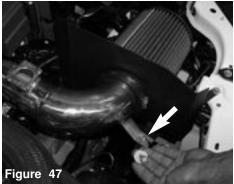
Use the m6 flange nut and fender washer to fasten the intake bracket to the vibra-stud
