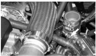
The 10mm crank case hose and the BOV straight hose are now installed.
