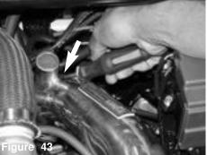
Use the 8mm press nut to tighten the clamp on the step hose.
