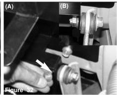
The m8 flange nut is used to secure the heat shield bracket to the air box brace (A). The m8 flange nut is tightened on the 12mm bolt (B).
