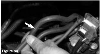
Align the upper vacuum line to the secondary intake vacuum port.
