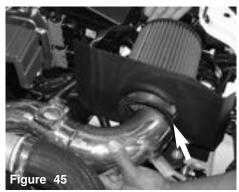
The filter neck base is pressed over the inlet side of the intake.
