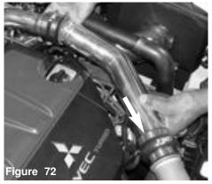
Insert the remaining tube into the hump hose as shown above.
