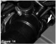
The clamp on the air intake duct that connects to the turbo inlet is loosened.
