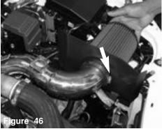
Once the filter stops are butted up against the rim of the intake, continue to tighten the filter neck clamp.
