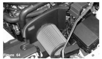
The vinyl trim is now installed over the heat shield edge.
