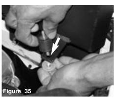
The m6 vibra-mount is inserted into the hole located on the heat shield bracket. The m6 flange nut and fender washer are used to fasten the vibra-mount to the bracket.
