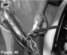
Press the 10mm hose over the intake vacuum port until it covers 75% of the vacuum port.
