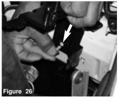
The 4th and final 12mm bolt is loosened and removed from the bottom of the air box bracket. The bolt is replaced to hold the new heat shield.
