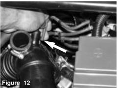
The second 4mm vacuum hose is now disconnected from the air intake port
