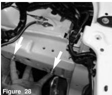
The bracket bolts that were removed in figure 24 are used in this picture, leave enough gap to slide the heat shield slots over the bolts.
