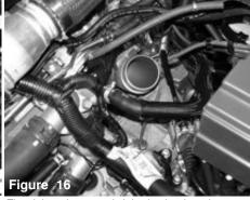
The air box cleaner and air intake duct have been removed and the turbo inlet is now exposed.
