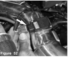
Align and connect the electrical harness to the mass air flow sensor.
