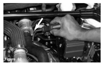
Once the BOV has been installed, continue to tighten the clamp on the straight hose.
