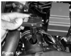
Once you have removed the stock bolts, continue to pull the mass air flow sensor from the sensor housing.
