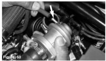
The 4mm vacuum line is pressed over the stock BOV port as shown above.
