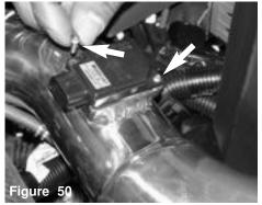
Fasten the mass air flow sensor to the machined adapter with the m4  $\times$  10mm bolts.
