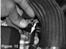
Disconnect the 10mm breather hose from the crankcase port as shown above.
