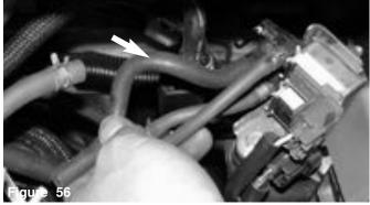
Align the lower 4mm hose over the intake port
