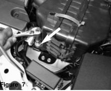
Loosen and remove the 10mm bolt that fastens the air box to the bottom bracket.
