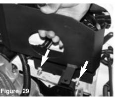
The heat shield is lowered and aligned to the two 12mm bolts.
