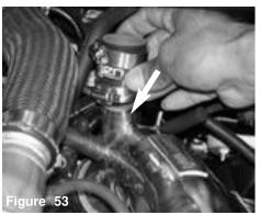
Press the 1 3/8" hose over the intake BOV port, place two small clamps on the hose, tighten the lower clamp over the BOV hose.
