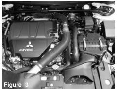
Stock air intake cleaner and upper intercooler piping shown in this picture
