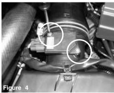
The stock bolt are removed from the mass air flow sensor as shown above.
