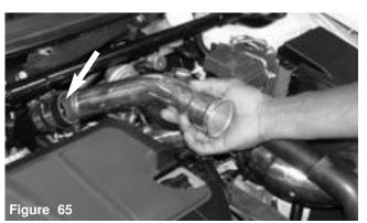
Insert the upper 2" intercooler tube into the upper 2" inlet.
