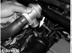
Now that the BOV clamp is loose, continue to pull the BOV from the air intake port.
