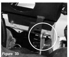
The 12mm bolt and flange nut secures the heat shield bracket to the stock air box brace.
