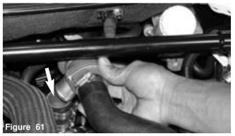
Once you have connected the 4mm vacuum line, continue to insert the BOV into the straight hose as shown above.
