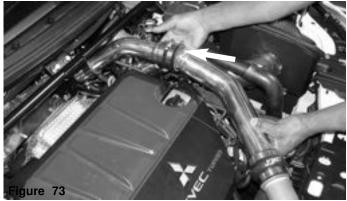
The upper end of the 2 1/2" tubing is pressed into the connecting 2 1/2" " hose on the upper intercooler tubing. Align for best fit and continue to tighten the clamps.
