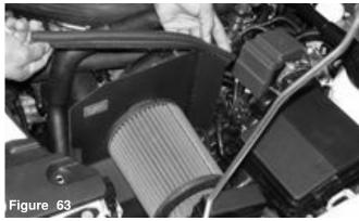
Align and press the vinyl trim over the edge of the heat shield.
