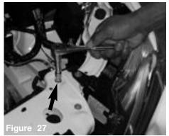
The corner cross member 10mm bolt is removed in order to attach the heat shield bracket later in the instructions.
