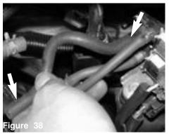
The 6" -4mm hose is pressed over the lower solenoid port.
