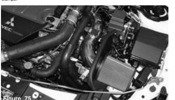
Top shot of the complete installation without the intercooler piping.
