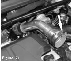
Once the hose has been installed, continue to tighten the clamp over the tubing.
