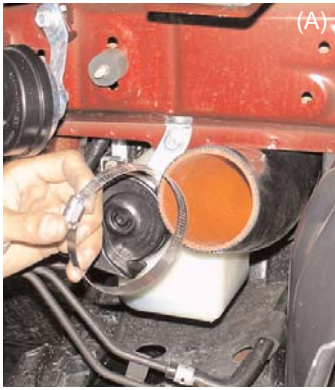
Take the medium clamp and locate it over the end of the silicone intake (A). Take the coupler with bracket and press it into the silicone intake (B).
