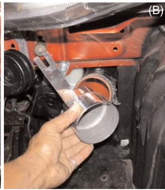
Take the medium clamp and locate it over the end of the silicone intake (A). Take the coupler with bracket and press it into the silicone intake (B).
