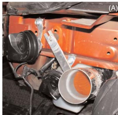
Once the coupler has been pressed into the silicone hose, align the coupler bracket to the vibra-mount stud (A). Place the fender washer and m6 flange nut over the vibra-mount stud and use the 10mm socket to fasten the flange nut to the vibra-mount stud (B).
