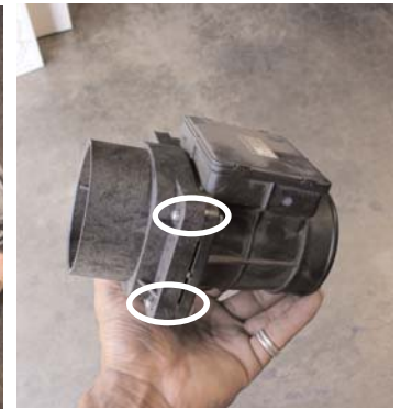
Take the finned composite flange, butt it up to the flat surface of the MAFS. Use the 4- 6mm flange nuts to bolt the flange to the MAFS.
