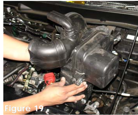
Figure 16 Now that all clamps on the air intake duct are loosened, continue to remove the air duct from the throttle body and air box cleaner.
