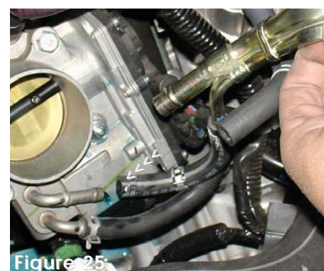
Figure 22 The tension clamp is depressed on the coolant outlet hose and pulled back.
