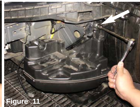
Figure 11 Remove the second 10mm bolt. Now the air resonator box is ready for removal.
