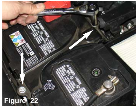
Figure 23 Now remove the battery tie down.
