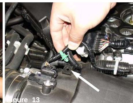
Figure 13 On top of the factory air box, you will need to unclip the green retaining clip attached to the air mass sensor harness.
