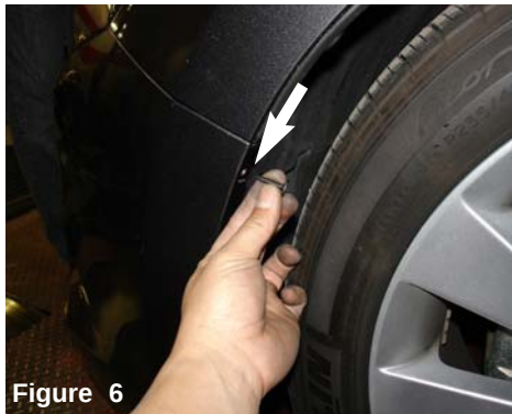
Figure 6 Picture shows removing phillips screw from bumper
