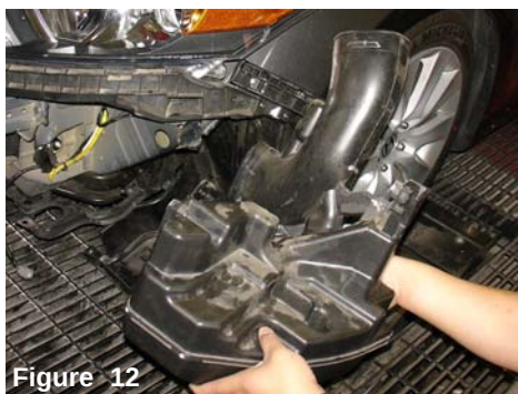
Figure 12 Firmly pull down and out to remove air resonator box. This may require some aggressive pulling when removing the resonator box.
