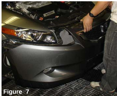
Figure 7 Firmly pull the sides of the front bumper outward until the bumper unlatches from the clips located below the headlights.
