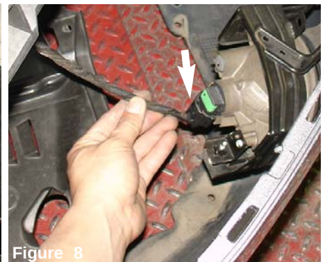
Figure 8 Pressing down on the center tab, unclip the fog light harness from the fog light bulbs on the passenger side and driver side bumper. Passengers side is shown above.
