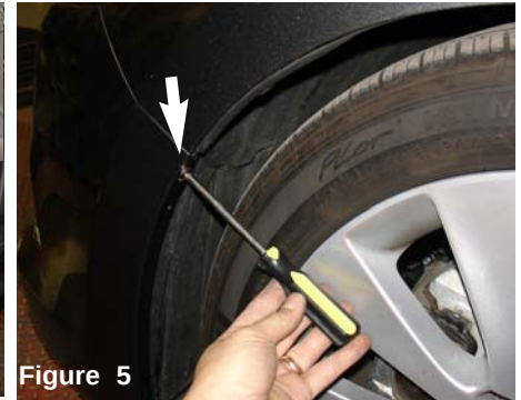
Figure 5 Remove one phillips screw on each side of the front bumper using a phillips screw driver
