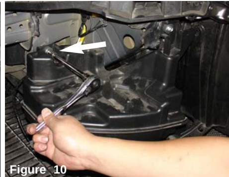
Figure 10 With the front bumper removed, you can now access the air resonator box located on the driver side. Use a 10mm 3/8 socket and ratchet to remove one 10mm bolt.
