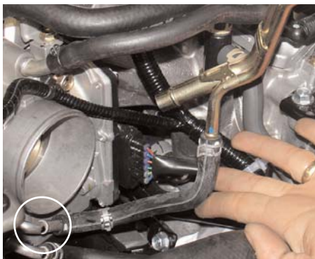
The last coolant hose is disconnected from the throttle body coolant inlet port.
