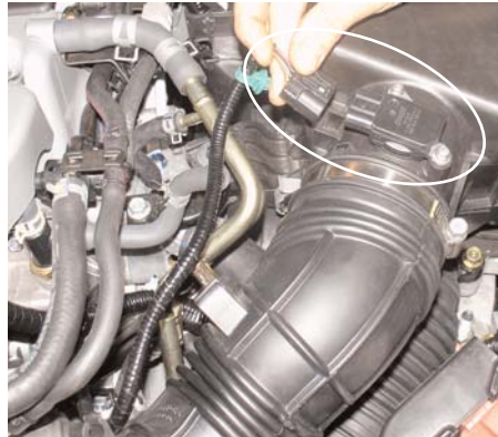
The harness clip is removed from the mass air flow sensor.
