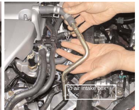
The larger PCV hard line connects the short hose on the crankcase to the air intake box. Next, disconnect the PCV pipe at the crankcase hose.
