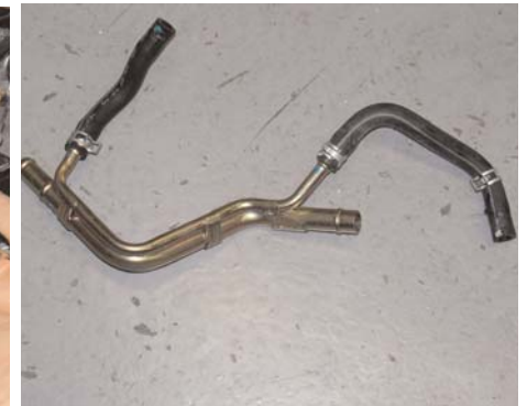
The PCV hard pipe is now removed from the engine compartment intacted.
