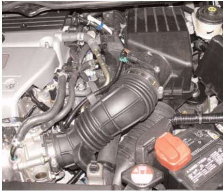
Stock air intake box ready to be removed from the engine compartment.
