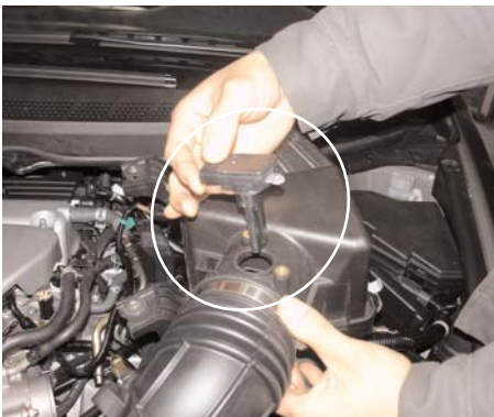
Remove the two screws holding the mass air flow sensor to the air intake duct. Gently, pull the mass air flow sensor from the air intake box as shown above.
