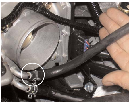
Insert the other end of the 6mm vacuum hose over the throttle body coolant port as shown above. Use the stock clamp to secure the hose over the port.
