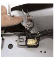
Take the assembled grounding wire and bolt and place it in its new location as shown above.
