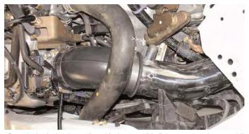
Once the intake has been aligned for best possible fit have a second person shift through all the gears to make sure that the intake does not obstruct the shifting in anyway. If the lever does not hit the intake continue with the installation of the intake.
