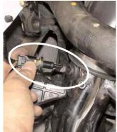
Locate the air temperature sensor and press it into the 1525 sensor grommet.
