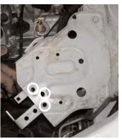
will need a drill and a 3/8" drill bit to drill three hose on the spot welds that holds the bracket in place
