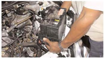
Remove the stock battery tie down and remove the cables from the battery. When safe to do so, remove the battery from the engine compartment and place it on a table or cardboard.
