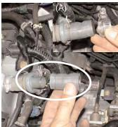
Remove the short stock hose (A) that connected the crankcase port to the air box as shown in this picture.
