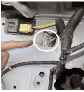
Using a 10mm socket or nut driver remove the ground wire bolt from its stock location.
