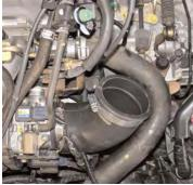
Take the 65 degree silicone elbow and place the 2 7/8" side over the throttle body. Use two clamps in this kit to place them on each end of the elbow.
