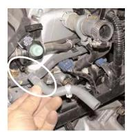
Remove the remainder of the thermal valve bypass control hose from the intake port.
