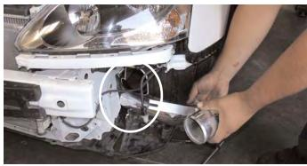
Install the upper portion of the intake through the bumper opening. Bring it up into the engine compartment and into the throttle body elbow.
