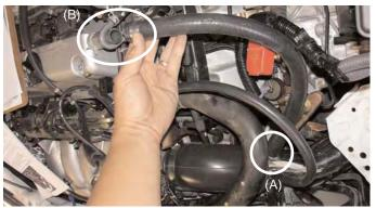
Take the 18" 17mm vacuum hose and press one end over the 3/4" intake port (A). Press the other end over the crankcase port (B), use the small clamps in this kit to secure the hose at the crankcase and the intake port.
