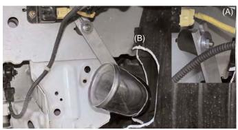
While the upper end has been inserted into the silicone elbow, align the intake bracket to the vibra-mount stud (A). Use the m6 flange nut and fender washer to secure the intake in place. The filter end of the intake should be positioned as shown in the picture above(B).
