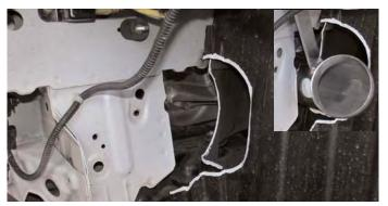
Cut an opening in the plastic splash guard as shown in the picture above. The side top portion has two sides that will require cutting in order to insert the cold air intake. Enlarge the opening as needed by fitting the filter end of the intake into the opening.
