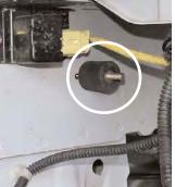
Take the 6mm vibra-mount and place it in the location where the grounding wire was originally removed from.
