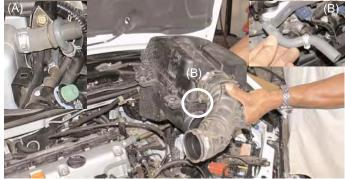
Remove the two bolts that secure the engine cover. Use a pair of pliers to depress the hosel clamp at the crankcase(A). Now depress the clamp on the air temperature sensor and remove it from the stock intake tube, do the same for the thermal valve vent hose(B). Remove the five bolts that secure the air intake box and pull the box up and away from the engine compartment.
