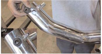
Take the 1525 sensor grommet and press it into the pre-drilled 3/4" hole as shown in (A). Insert the grommet into the hole until grommet is well seated throughout the hole circumference.
