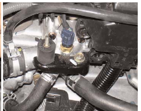
Screw the vibra-mount firmly into the brace until it sits flush on the brace.
