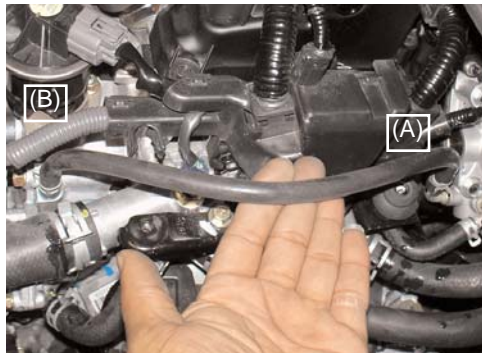
The 15"-6mm vacuum hose is now connected from the throttle body (A) to the upper coolant outlet port (B).
