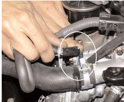
Remove the stock upper coolant outlet hose pressed over the port as shown above. Place finger over the port to prevent coolant from spraying out.
