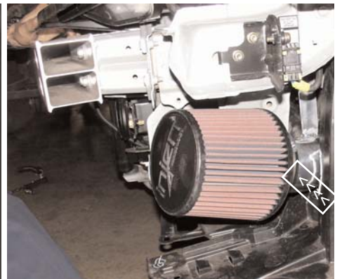
Press the filter over the end of the secondary intake and tighten the clamp on the filter neck. You have now completed the installation of this intake system.
