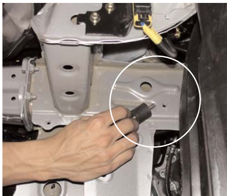
The secondary vibra-mount is aligned and screwed into the pre-tapped hole located on the side frame.
