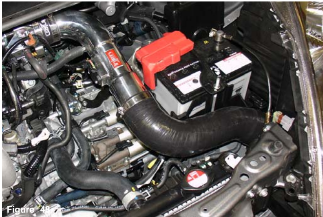
Figure 48 Align the entire intake for the best possible fit. Once the intake has been cleared from all moving parts, continue to tighten all nuts, bolts and clamps. Periodically, check the fitment of the entire intake to prevent damage to the intake.
