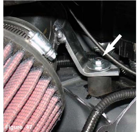
Figure 47 The m6 flange nut and fender washer is tightened over the vibra-mount stud.
