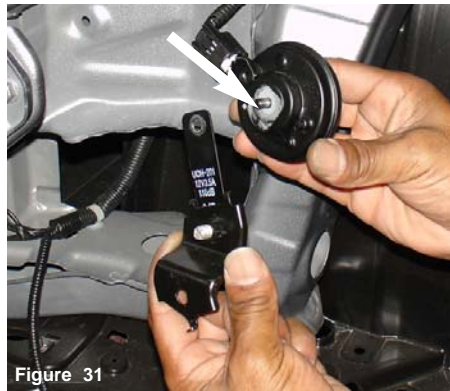
Figure 31 Once the horn has been removed, continue to removed the nut holding the horn and bracket together. Separate the horn from the bracket.
