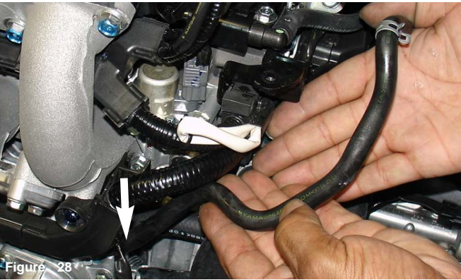
Figure 26 The breather hose coupler is pulled from the crankcase port (A). The line connected to the upper intake manifold port is also removed (B).
