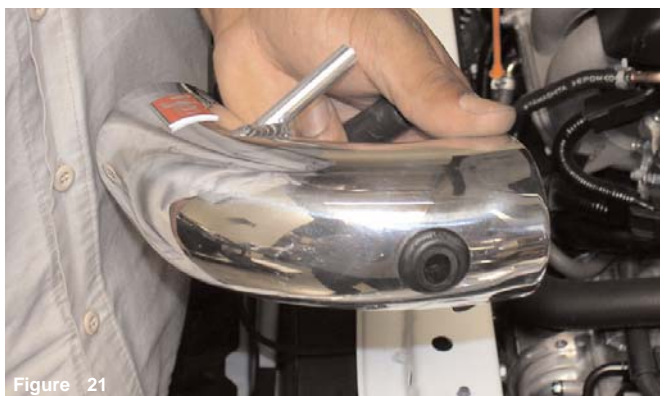
Figure 21 The sensor grommet is now sitting flush in the pre-drilled intake hole.
