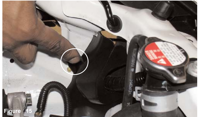
Figure 15 The second plastic clip is removed from the fender wall area.
