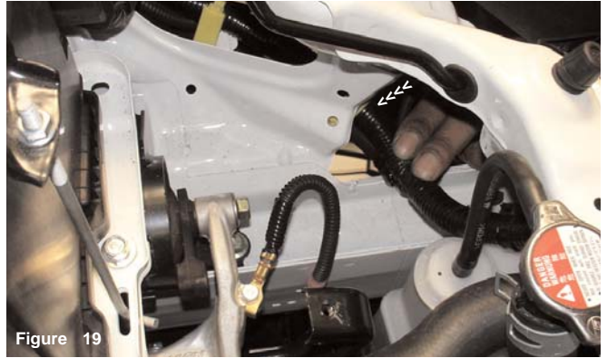
Figure 19 The harness is pulled away from the fender until a clear path has been created for the silicone intake.
