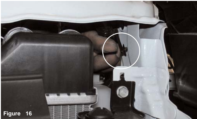
Figure 16 The inner plastic plug is removed from the main frame support.
