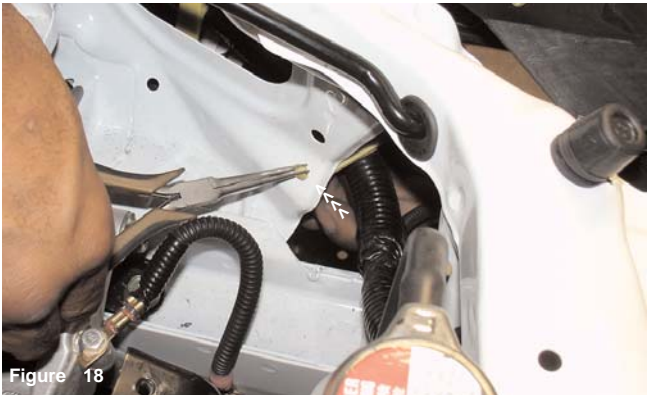
Figure 18 The harness clip is compressed and push through the fender in order to free the electrical harness.
