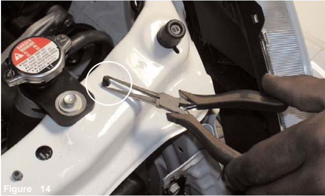
Figure 14 The first top clip is removed by compressing the tabs and pressing the pin through the hole.
