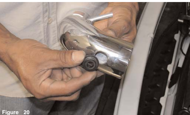
Figure 20 Insert the 1560 grommet into the pre-drilled hole located on the intake.
