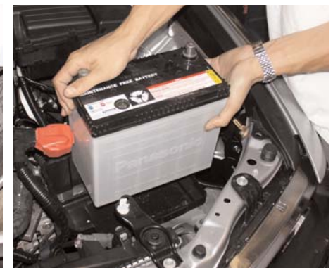
For best positioning of the cold air intake, removal of the battery will be required.
