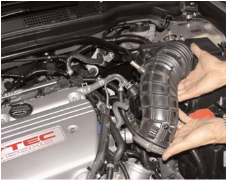
Loosen clamps and remove the air intake duct as shown above.
