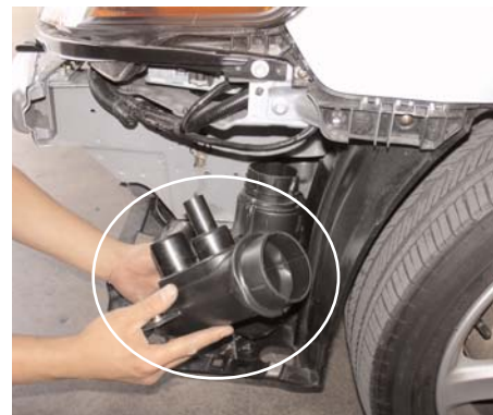
With the air resonator box out, remove the resonator connecting duct that connects the air resonator tube and air resonator box.
