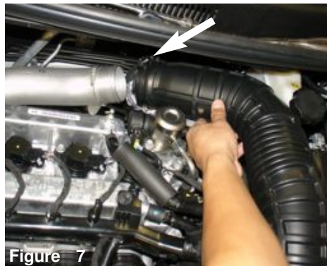
Figure 7 Use a 10mm socket and ratchet and loosen the 10mm clamp bolt on the air duct located on the Turbo charger compressure outlet. Pull the air duct from the outlet.
