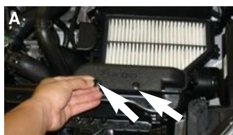
Figure 7 Use a 10mm socket and ratchet and loosen the 10mm clamp bolt on the air duct located on the Turbo charger compressure outlet. Pull the air duct from the outlet.
