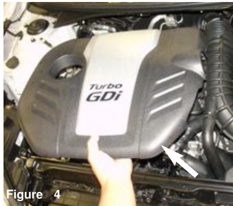
Figure 4 Firmly lift up on the engine cover and remove the engine cover from the engine bay.
