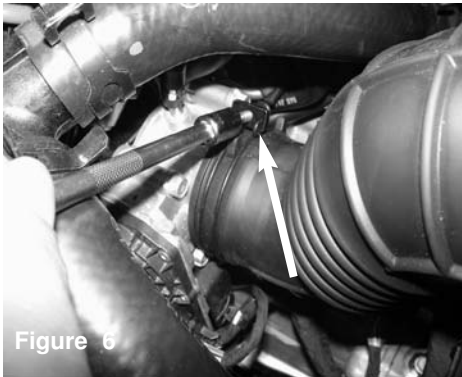
Figure 6 Use a 10mm socket/ratchet loosen the clamp in the throttle body.
