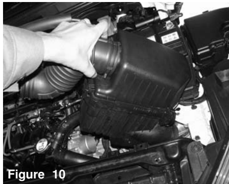
Figure 10 Now carefully lift up and remove the complete air box assembly from the vehicle.
