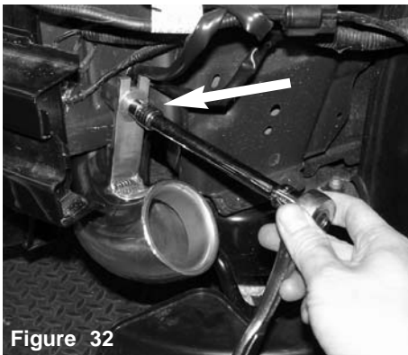
Figure 30 With the intake pipe in place, make sure the lower intake bracket lays flush with the vibramount
