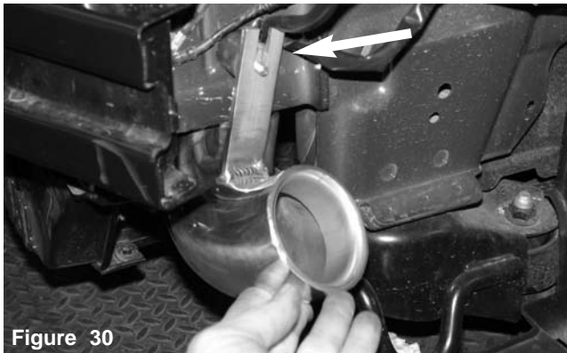
Figure 28 Slide the intake pipe from the bottom and work the pipe into the 90 deg. hose already located on the throttlebody.
