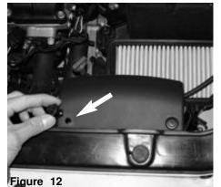
Once you have loosened the center screw on the clip, continue to pull the clips out.
