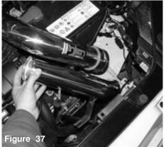
The secondary intake is now lowered into the driver side corner bumper.
