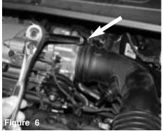
Loosen the air duct clamp located over the throttle body.
