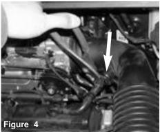
Compress the tension clamp and retract it away from the vacuum port.
