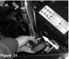
Converting the intake into a cold air intake, aligned and slip the 2 3/4" hose over the end of the intake.
