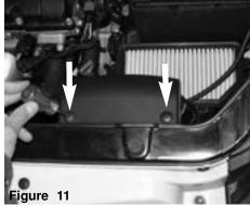
Loosen the two screws located on the front air scoop.
