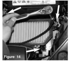
The first of three bolts are loosened from the lower air box as shown above.
