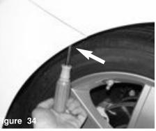
The bumper corner screw is loosned and removed in the wheel well.
