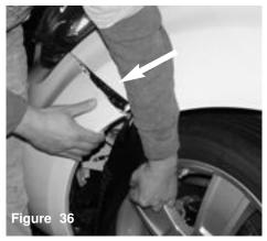
The mudd guard and the corner bumper are both separated in order to make room for the filter.
