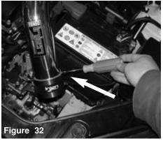
The clamp hose over the intake end is now tightened.
