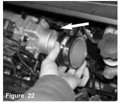
Thefirst 2 3/4" straight hose is aligned to the throttle body as shown above.
