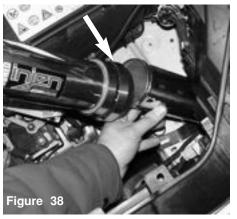
The primay intake end the the secondary are conneted to each other.
