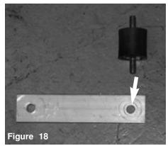
The first vibra-mount is aligned to the bracket as shown above.
