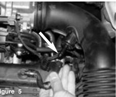
Once the tension clamp has been removed continue to remove the vacuum line from the intake port.
