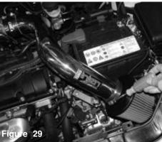
The filter is aligned over the end of the primary intake. Once the intake is resting against the filter stops the filter clamp is tightened as shown above,
