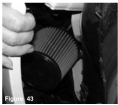
Once the filter stops come to rest over the intake end, continue to tightened the filter neck.
