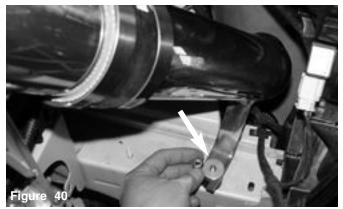
The m6 flange nut and washer are placed over the vibra-mount stud and tightened.
