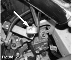
As the upper intake is inserted into the throttle body hose, The intake bracket is aligned to the vibramount stud.
