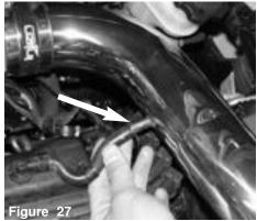
The stock crankcase vacuum line is re-aligned to the intake vacuum port.
