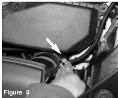
Unlatch the two clips holding the upper air box to the lower box. The first metal clip is unlatched.
