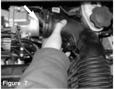
Once you have loosened the clamp, continue to detach the air duct from the throttle body.
