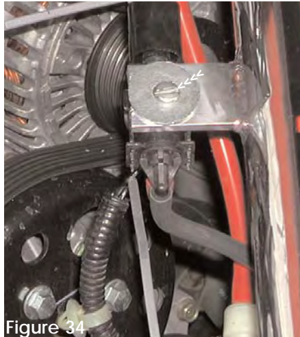
Figure 31 Press the stock air injection pump line over the 3/4" intake port.
