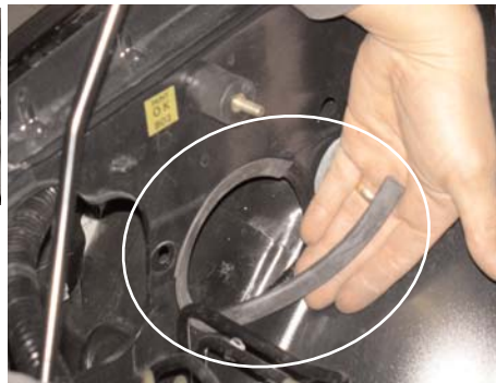
Use the 12" vinyl flex trim to align the resonator opening. The entire resonator opening must be covered to prevent the edge from cutting into the intake.
