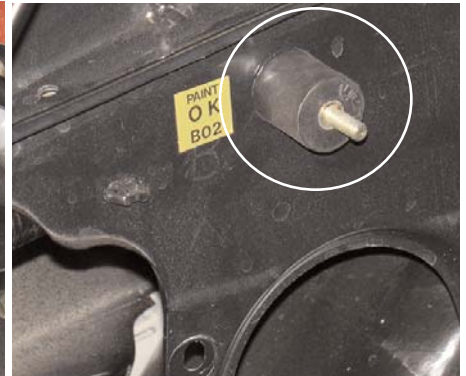
The vibra-mount is screwed into the fender wall just above the round resonator opening. The vibra-mount is screwed in until it bottoms out.
