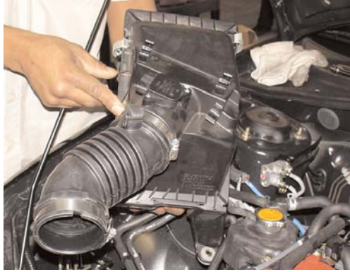
Loosen all clamp, then remove the entire air intake box and the air intake duct all in one piece.
