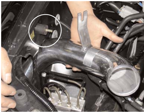
Insert the secondary intake in the resonator opening and align the intake bracket to the vibra-mount stud.
