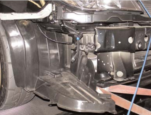
The front bumper and air intake resonator has been removed for installation of the cold air intake.
