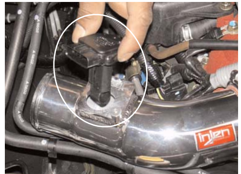
Insert the MAF sensor into the machined sensor adapter and use the same stock screws to secure the sensor in place.
