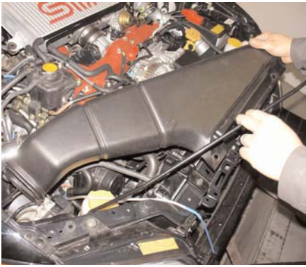
Remove air scoop from the top cross member and resonator opening.
