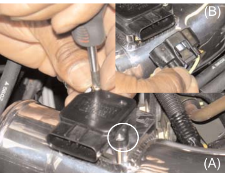
Use the stock screws to fasten down the mass air flow sensor (A), continue to press harness clip over MAF sensor until you hear it snap in place (B).
