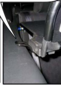
STEP 1: YOUR LOVE THE DRIVE WIND DEFLECTOR ATTACHES TO THE SMALL HOLES IN THE TRIM PANEL. YOUR WIND DEFLECTOR HAS TWO "L" HANDLE SPRING PLUNGERS. THE "NOSE" OF THE PLUNGERS WILL GO INTO HOLES. START WITH THE PLUNGERS IN THE CLOSED POSITION, AS IN THE SECOND PICTURE.
