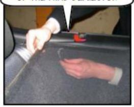
STEP 3: LOWER YOUR WIND DEFLECTOR SO THE "NOSE" OF THE PLUNGER IS IN LINE WITH THE HOLE IN THE TRIM PANEL
