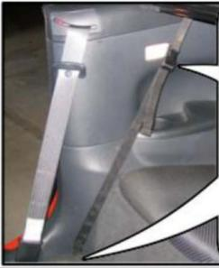
STEP 5: THERE ARE TWO FRONT STRAPS. THESE STRAPS ATTACH TO THE BOTTOM OF THE TRIM PANEL (BELOW THE BACK SEAT) AND THEN TO THE BUCKLE UNDER THE FRONT BRACKETS. REPEAT ON THE OTHER SIDE.
