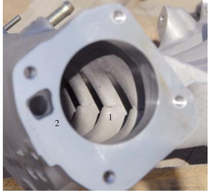
Clone Manifold: 1) has rough transitions from plenum to runners and horrible parting lines which is a result of poor design and careless manufacturing. 2) Standard size IAC opening and passageway can only accommodate throttle bodies up to 66-68 mm. User won't be able to properly port match and blend opening back into plenum without breaking through the IAC passage.
