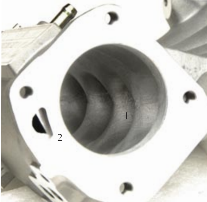
Skunk2 Manifold: 1) has smooth transitions from plenum to runners and clean parting lines. 2) IAC opening and passage way has been reduced to accommodate larger throttle bodies up to 75mm. User will easily be able to port match opening and smoothly blend back into the plenum without the risk of breaking through the IAC passage.
