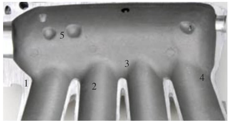
Clone Manifold: 1) Abrupt transition from throttle body to runner #4, 2) transition between runners is more square, notice how runner entry is straight. Some runner entries are even pinched off/ reverse tapered (especially 2 end runners). 3) Abrupt transitions between plenum and runner; that is why there are distinct dark shadows. 4) Abrupt transition from end of plenum to runner #1. 5) Unnecessary protrusions into plenum to accommodate IAC bolts.
