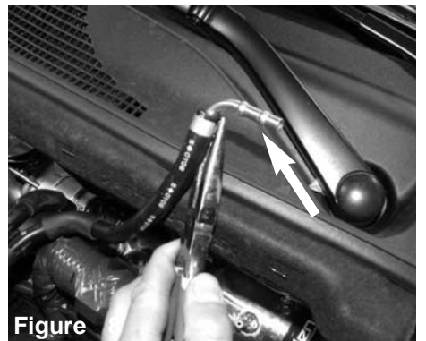
Figure 5 Install the 2-3/4" straight hose with clamps provided to the intake tube. Do not tighten.
