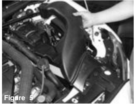
Figure 5 Once you have removed the two plastic clips, continue to remove the front air scoop.
